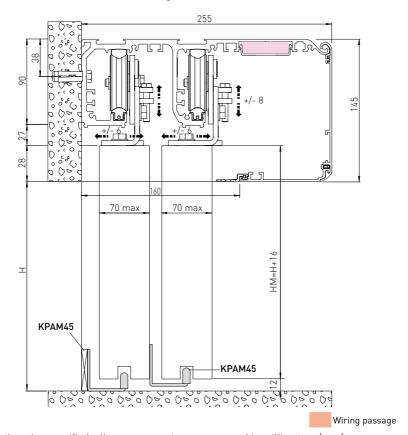
Unless otherwise specified, all measurements are expressed in millimetres (mm).
