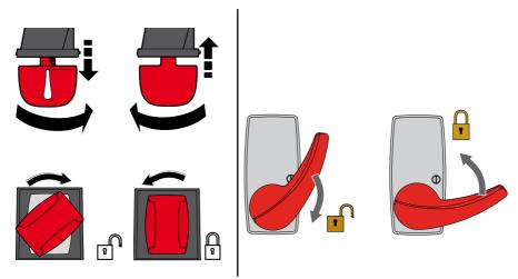
In the event of maintenance, malfunctioning or emergency, pull the lock release lever VALSB down and turn it to the right or lower the lock release lever LOKSBM (if installed) and move the door wings manually into the open position.
